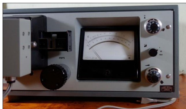
Fig 1: UR-20 Carl Zeiss Jena spectrometer
