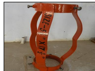
Fig 2: Welded semi rigid type centralizer
